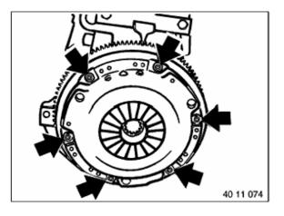
Release screws 1 turn in diagonal sequence until tension is relieved on clutch cup spring.
