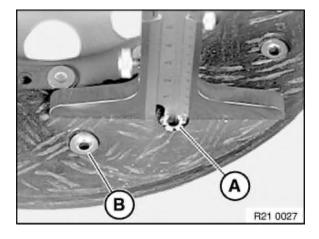
Checking clutch plate for wear:
